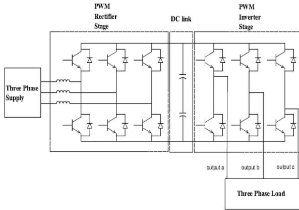
Fig. 5.1: Schematic of AC to AC converter.
