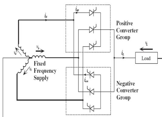
Figure 3.1 Single-phase load fed from a three-pulse cycloconverter.
