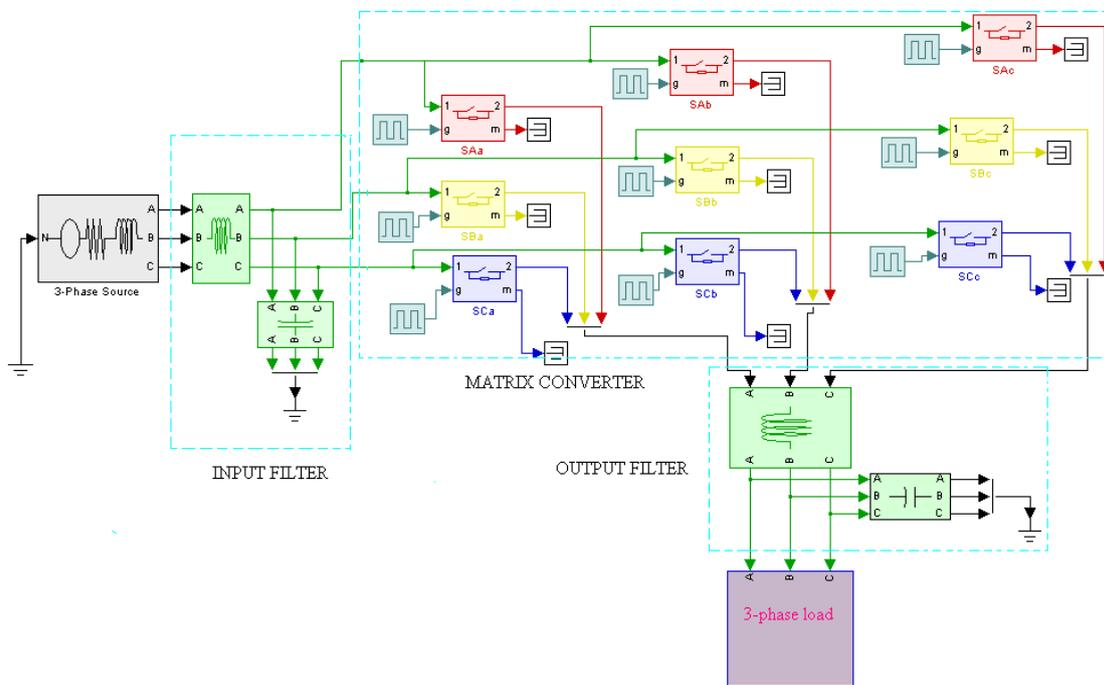
Figure 4.1: Schematic of Matrix Converter used in MATLAB simulation.
