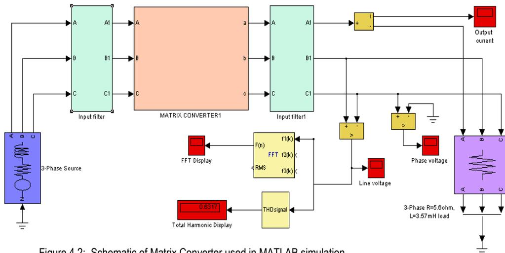
Figure 4.2: Schematic of Matrix Converter used in MATLAB simulation
