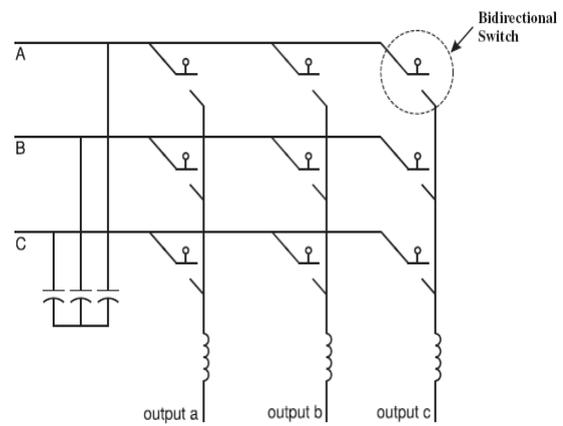
Figure 1.2: Structure of Matrix Converter.
