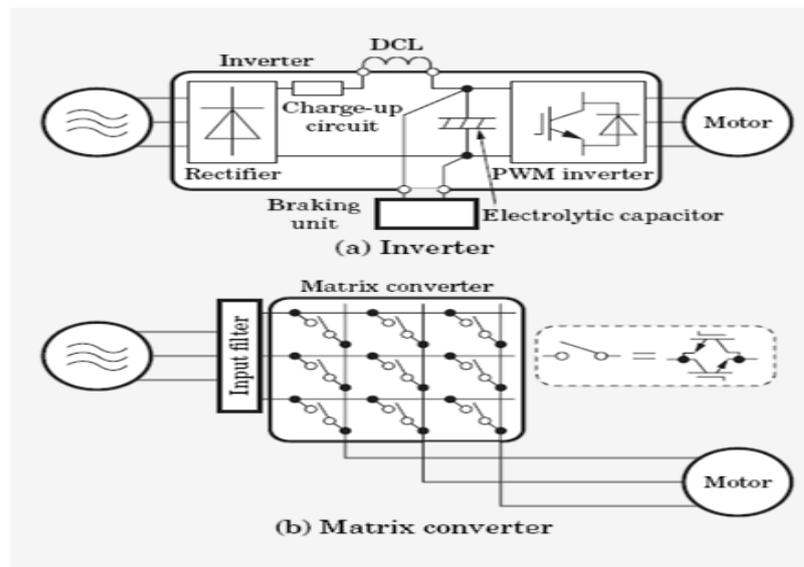
As can be seen in Figure 4.1, the inverter required a charge up circuit to suppress the inrush that flow to electrolytic capacitor connected to DC link circuit. If a diode rectifier is used for converting AC voltage into DC voltage, a large amount of input current harmonics will be generated and therefore, a DC reactor (DCL) is inserted to reduce the harmonics in the input current.
