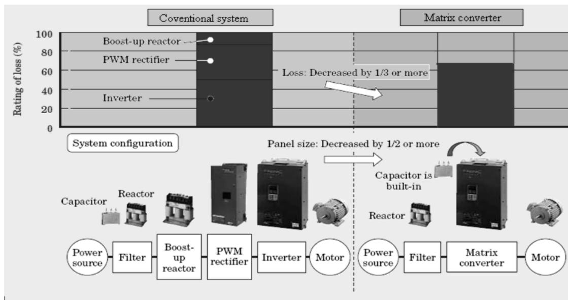
Figure 4.2 Comparison of the matrix converter with the conventional system
