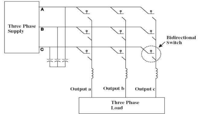
Fig. 5.2: Simplified representation of a Matrix Converter system.
